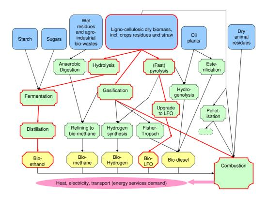
Figure I UK-MARKAL (MED) simplified bioenergy chains, with gasification, lignocellulosic bioethanol and fast pyrolysis bio-oil highlighted.
