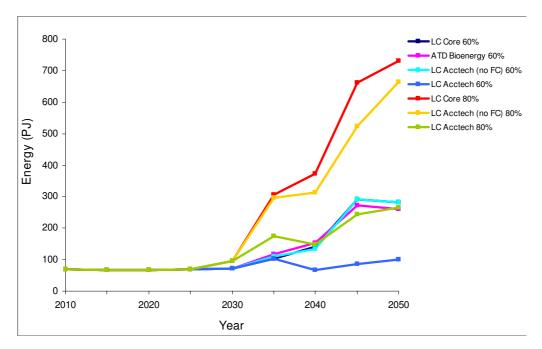
**Biomass for transport (biofuels) in the aggregate scenarios**. LC-Core (60%) (dark blue); accelerated technology development bioenergy (ATD Bioenergy (60%)) (purple); LC Acctech without fuel cells (60%) (LC Acctech (no FC) 60%) (aqua); LC Acctech with fuel cells (60%) (LC Acctech 60%) (blue); LC-Core (80%) (red); LC Acctech without fuel cells (80%) (LC Acctech (no FC) 80%) (yellow); LC Acctech with fuel cells (LC Acctech 80%) (green). Percentage value corresponds to carbon reduction targets.
