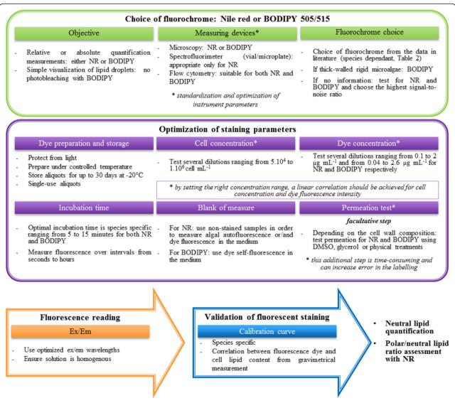
**Figure 1 General flow chart of an optimal protocol for lipid quantitative measurements in microalgae cells.** Setting of fluorescent measurement procedure exposed different steps from choice of fluorochrome to neutral lipid quantification with operational indication for both Nile red (NR) and BODIPY 505/515 (BODIPY). DMSO, dimethylsulfoxide; Em, emission; Ex, excitation.
