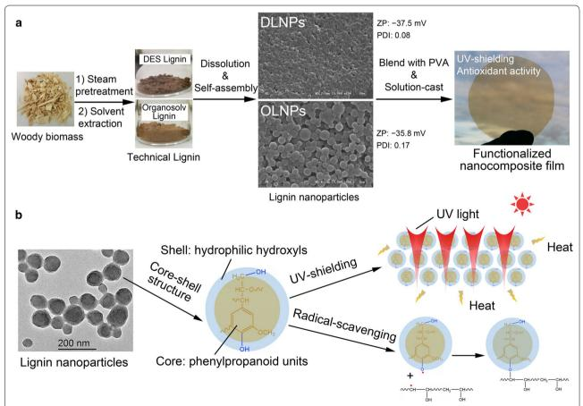
Fig. 1 a Synthetic procedure to fabricate lignin nanoparticles and the lignin nanoparticles/PVA composite film. ZP Zeta-potential value, PDI polydispersity index. b Proposed mechanism for UV-shielding and antioxidant activity using lignin nanoparticles as the functional additive
