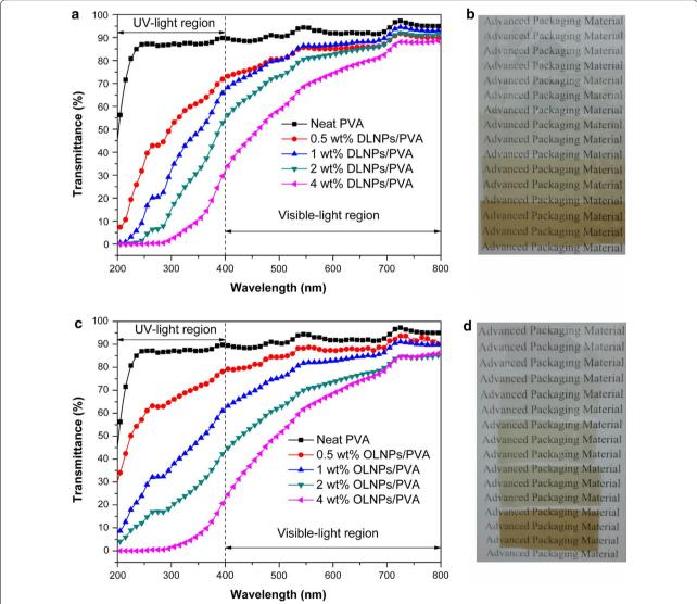
Fig. 2 UV–Vis light transmittance spectra and digital photographs of **a** and **b** DLNPs/PVA and **c** and **d** OLNPs/PVA composite films with 0–4 wt% lighin nanoparticles. The digital photographs show the high optical transparency of the lighin nanoparticles/PVA composite films (from *top* to *bottom*, the content of lighin nanoparticles in the film was increasing from 0 to 4 wt%)
