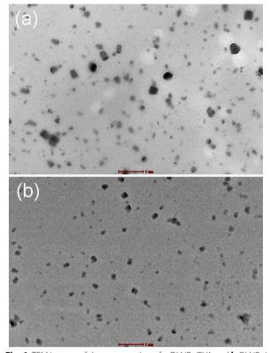
**Fig. 6** TEM images of the cross section of **a** DLNPs/PVA and **b** OLNPs/PVA composite film with 4 wt% lignin nanoparticles
