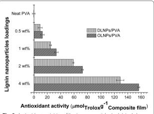
**Fig. 3** Antioxidant activities of lignin nanoparticles/poly(vinyl alcohol) (LNPs/PVA) composite films determined by TEAC assay
